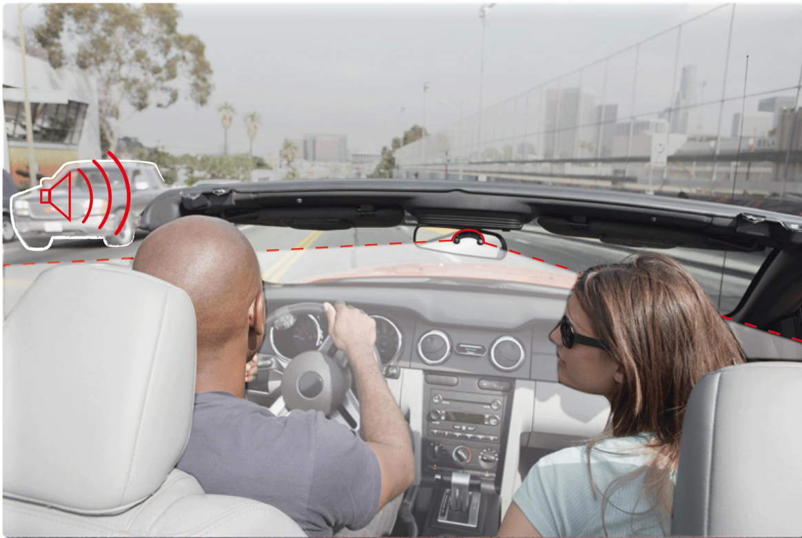
Lateral noise detection effect deactivated – Microphone misplaced
